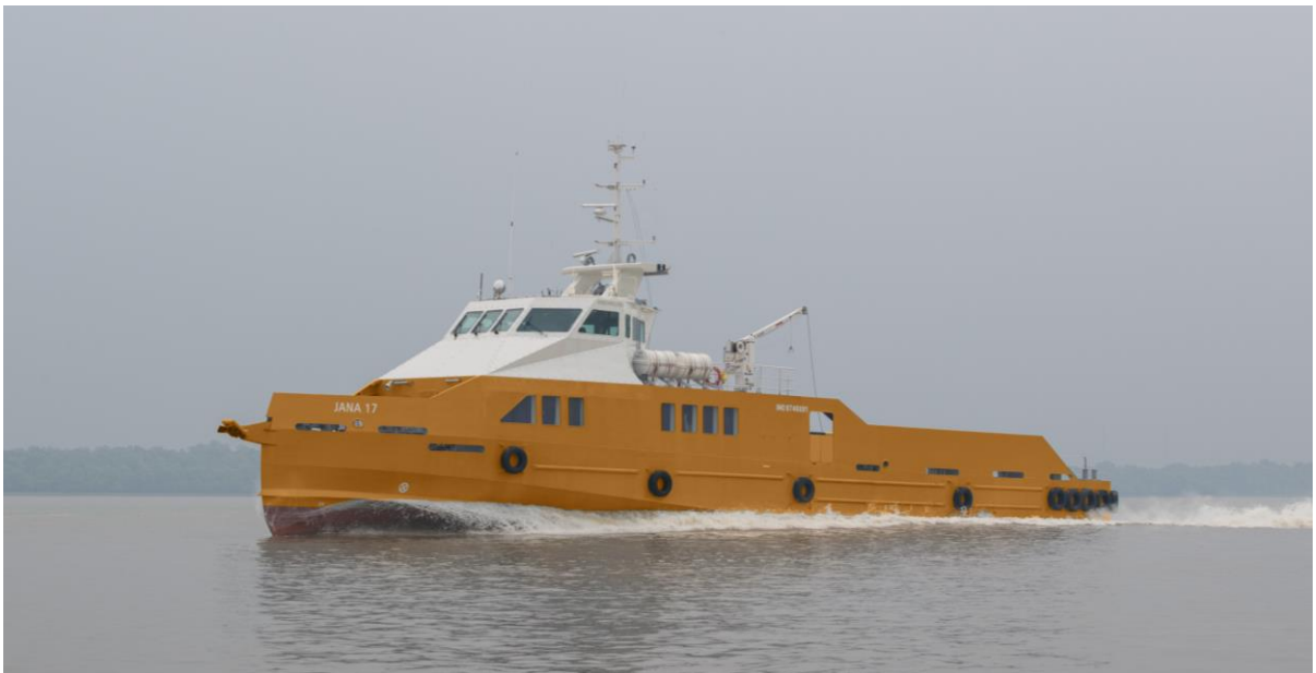
FPSV 41P: 41 m Fast Personnel and Supply Vessel / fixed pitch propellers
