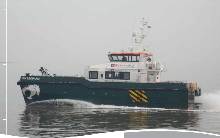
The PIRIOU WFSV 26P/w, based on a proven design by BMT Nigel Gee, benefits from PIRIOU's 30 years experience in delivering more than 100 aluminium crew boats to the offshore industry. The WFSV 26P/w is designed to ensure a fast, safe and comfortable transfer of personnel and equipment. This aluminium-built catamaran can carry 24 technicians, 4 crew (four twin cabins) and up to 3 standard 10 ft ISO containers.
