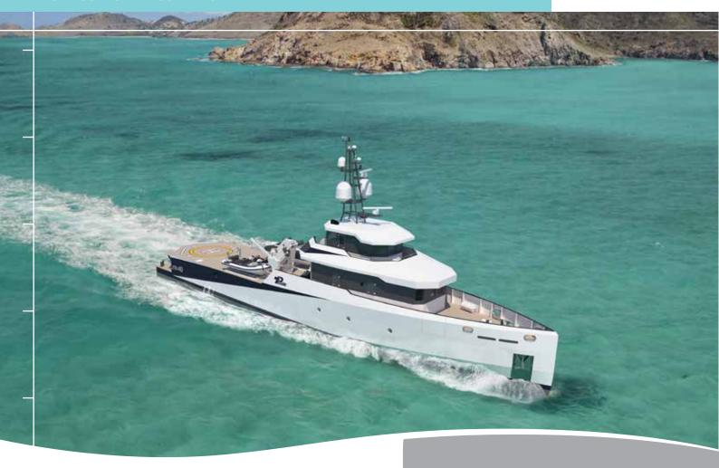
The PIRIOU YSV 40 is a rapid, ocean-going support vessel capable of carrying technical and leisure equipment for her mother yacht. Based on our Fast Passenger and Supply Vessel FPSV 40, her steel hull is suitable for all sea and weather conditions.
