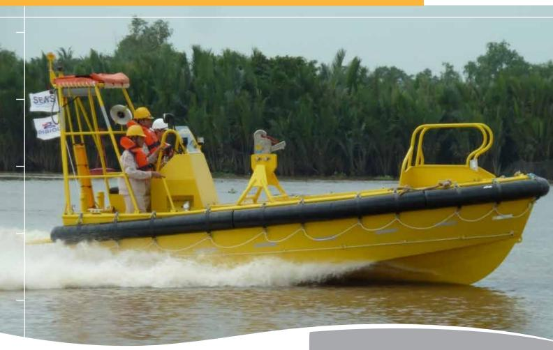
This Fast Rescue Boat originally designed for Offshore Support Vessels on board installation is also adapted to short distance crew transfers thanks to her standardized bow landing.
