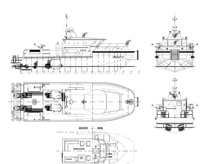
The FIRE 16 is designed to be a fire boat compliant to the National Fire Protection Association (NFPA) code, and stands as a very performing high speed craft
