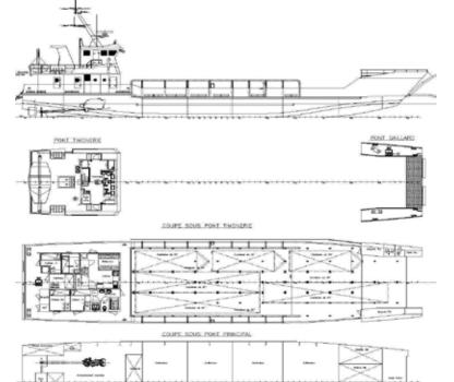
LCT cargo designed for loading and unloading by fore bow
