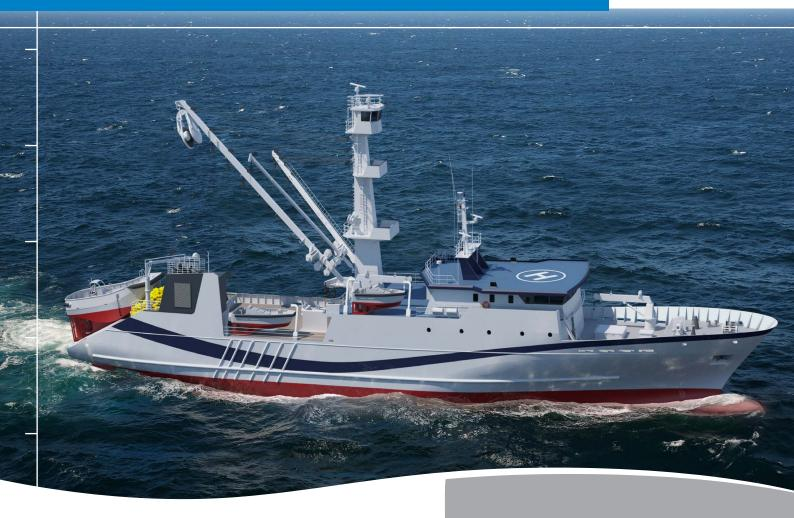
With over twenty five years experience of building oceanic and mediterranean tuna fishing vessels, PIRIOU has designed the PS 80-1620/1800, a performing and robust tuna seiner especially developed with versatile and modular equipment in order to adapt to all sorts of operation methods. She is 80 metres long and is especially fitted to West Pacific fishing.
