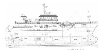
Deep freezer longliner designed for austral and antarctic pelagic fishing and fish conservation at - 25°C
