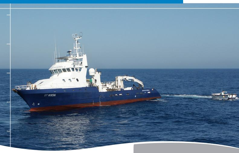
With over twenty five years experience of building oceanic and Mediterranean tuna fishing vessels, PIRIOU has designed the PS 36-205, a simple, robust and compact tuna seiner, especially developed for coastal fishing.
