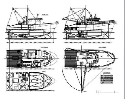
Shrimp freezer trawler designed for tropical shrimp fishing and its deep freezing at - 25°C
