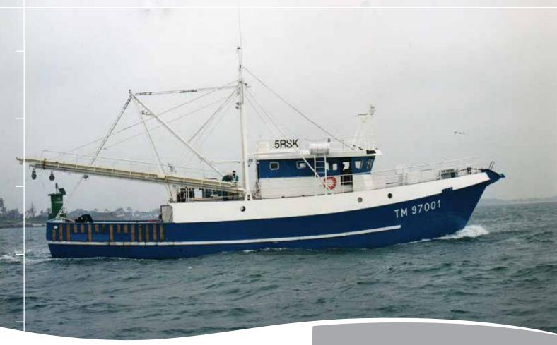
Shrimp trawler freezer designed for tropical shrimp fishing and its deep freezing at - 25°C
