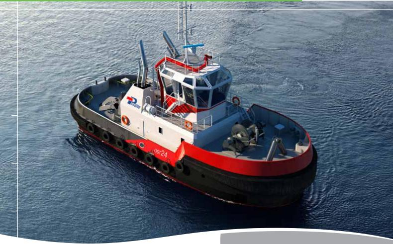
The OST 24 is the smallest model of the famous OST multipurpose harbour tug family designed by PIRIOU with a bollard pull up to 56 tons. These standard tugs are built in series for a shorter delivery time.
