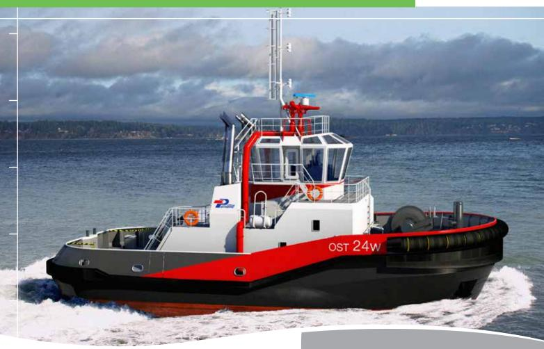
The OST 24 W is derived from the famous OST multipurpose harbour tug family designed by PIRIOU with a widened beam (W) for a bollard pull up to 74 tons. Medium speed engine variants are available for 45 and 65 tons bollard pull. These standard tugs are built in series for a shorter delivery time.
