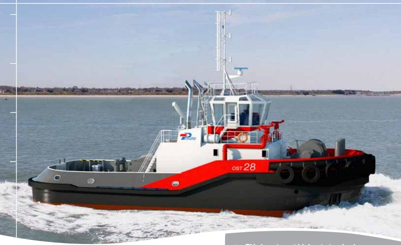
The OST 28 is part of the famous OST multipurpose harbour tug family designed by PIRIOU with a bollard pull up to 60 tons. These standard tugs are built in series for a shorter delivery time.
