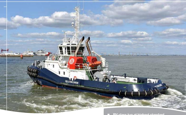
The OST 30 is the best seller model in the famous OST multipurpose harbour tug family designed by PIRIOU, with a bollard pull up range from 45 up to a powerful 74 tons. Medium speed engine variants are available for 45 and 65 tons bollard pull. These standard tugs are built in series for a shorter delivery time.
