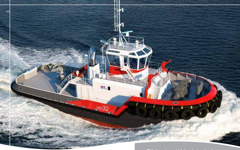
The OST 32 is the biggest model in the famous OST multipurpose harbour tug family designed by PIRIOU with a bollard pull up range from 72 up to a powerful 94 tons. The OST 32 can be offered either in medium speed or high speed engines up to 85 t BP. These standard tugs are built in series for a shorter delivery time.
