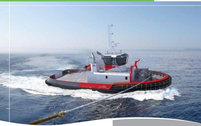
The OST 32 E is the latest addition to the famous OST multipurpose harbour tug family designed by PIRIOU with a bollard pull from 74 up to a powerful 94 tons. The OST 32 E can be offered either in medium speed or high speed engines up to 85 t BP. These standard tugs are built in series for a shorter delivery time.
