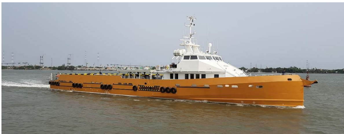
FPSV 55w: 55 m Fast Pax Supply Vessel with waterjets
