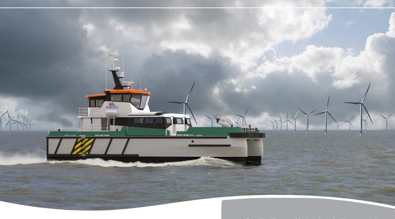
Developed internally, the 26m PIRIOU CTV benefits from previous Crew Transfer Vessels deliveries to the offshore wind industry and more than 100 crew boats built for the oil and gas sector.
