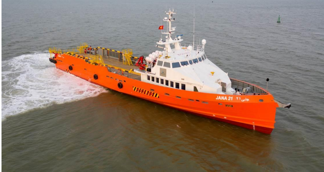
FPSV 55w: Fast Pax Supply Vessel de 55 m / hydrojets
