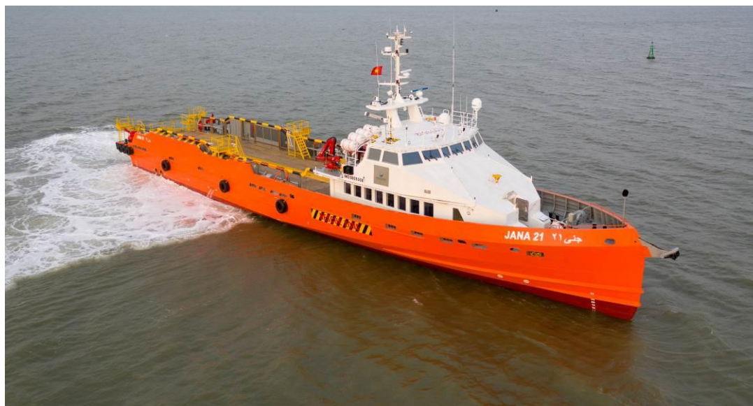
FPSV 55w: 55 m Fast Pax Supply Vessel with waterjets
